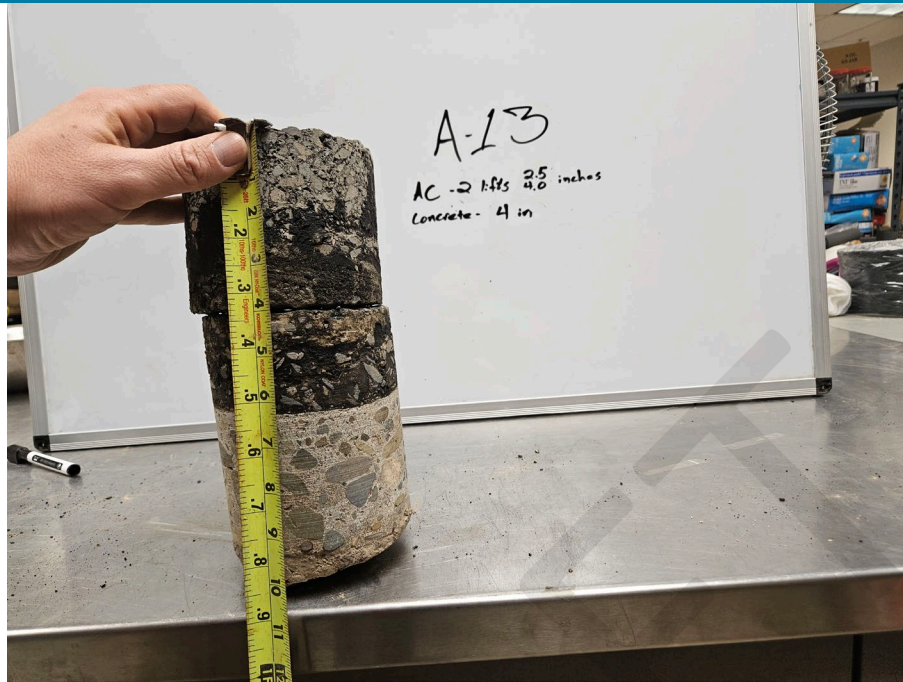
Photo 13: Pavement core from exploration location A-13.
