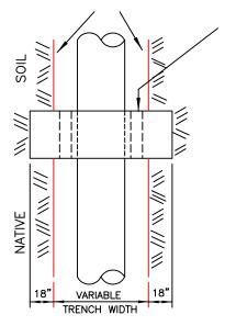
INSTALL 3" WEEP HOLES AT BOTTOM OF TRENCH WITH 1/4" GALVANIZED SCREEN OVER UPSTREAM END.
